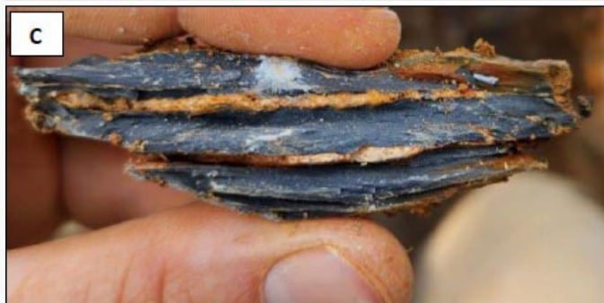
a) hand sample of fresh slate. c) hand sample of slate containing mm-scale foliation concordant stringers
